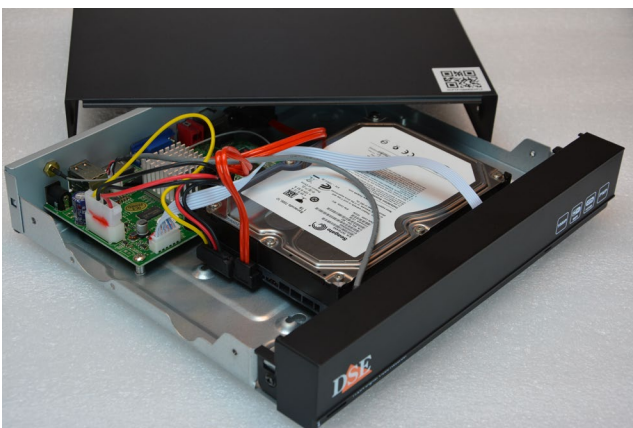
Secure the hard disk with the 4 screws provided screw from under the video recorder
